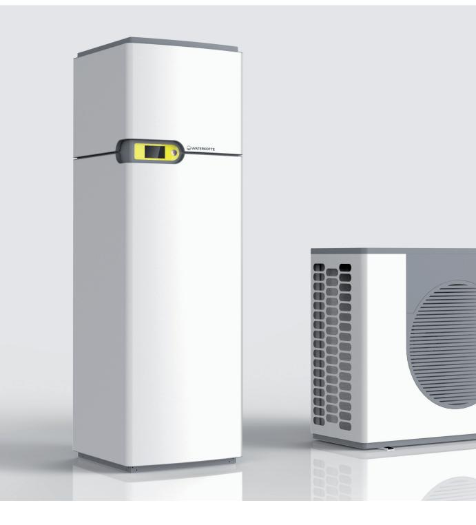
The new EcoTouch Ai1 Air uses the air as heat source. The system offers a complete solution in split design for low power requirements. The indoor unit is equal to the Ai1 Geo (see page 4|5). The newly developed outdoor unit is extremely economical. The compression performance adapts perfectly to the heat requirement by way of inverter technology. Thus, optimal efficiency factors and low operating
